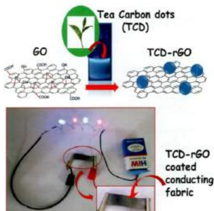
Fig. 2.4. Schematic Representation showing the process of fabricating conducting fabric.
