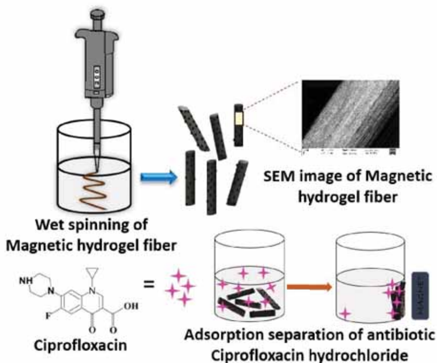
Fig.1 : Schematic representative showing synthesis of magnetic alginate- \text{Fe}_2\text{O}_3 hydrogel fibers by wet spinning technique and its use of adsorption / separation of antibiotic ciprofloxacin hydrochloride.
