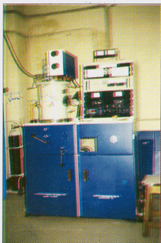
PLASMA PROCESSING CHAMBER WITH SPUTTERING UNIT
