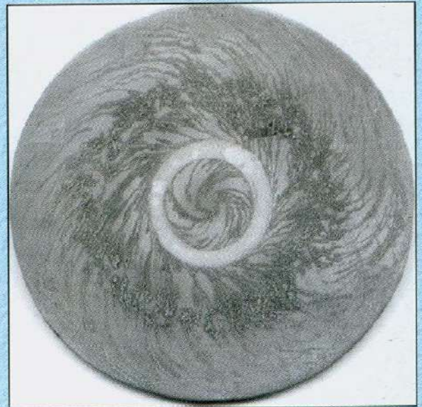
Sputtered commercial aluminium target in Planar RF Magnetron discharge
