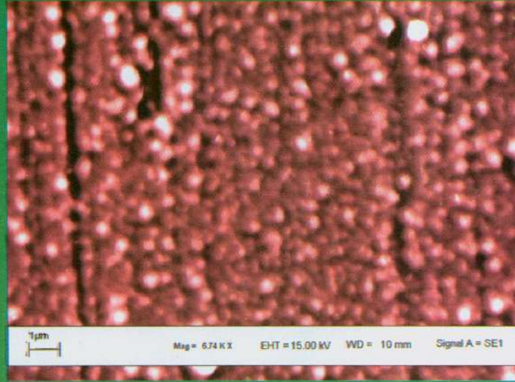
SEM of P 2 VP-Br 2 complex in nano fine state deposited at Polymer lab.
