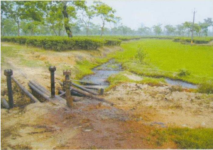
Photo.3. Contamination of Hydrocarbon in Tea garden due to spillage of Crude Oil from the pipeline of ONGC at Lakowa Oilfield GGS6
