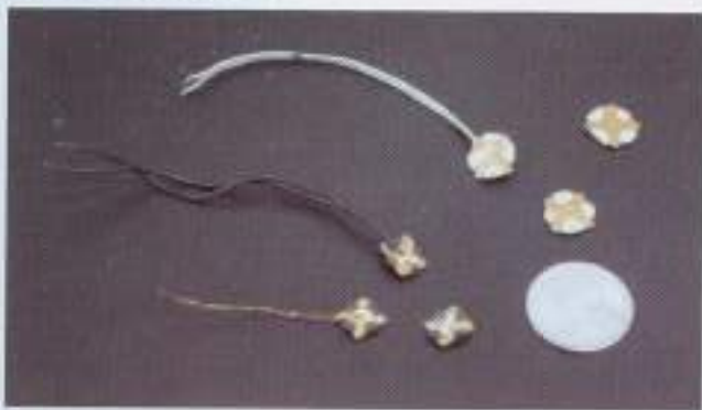
Figure 1.2.1. Thermistor devices of PCHMAS and PCHMASH
