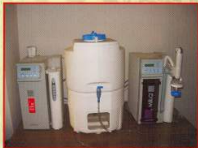
Milipore Water Purification System
