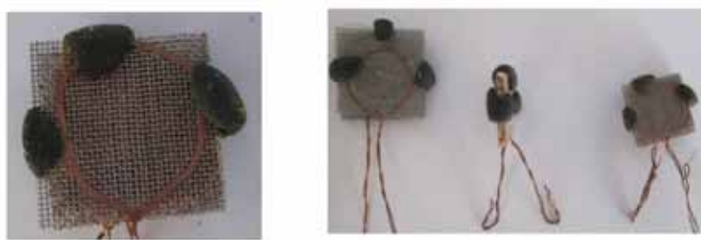
Figure 1: Fabrication of a trilayer detector
