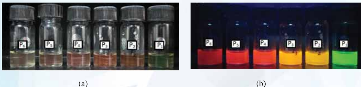
Figure 2. Photographs of the prepared QD samples under (a) normal light and (b) UV light (365 nm) samples P1 to P6 having different size QDs grown at different refluxing time.
