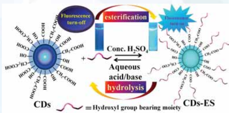
Figure 1: Schematic Representation of the reversible esterification-hydrolysis process exhibited by carbon dots derived from citric acid.
