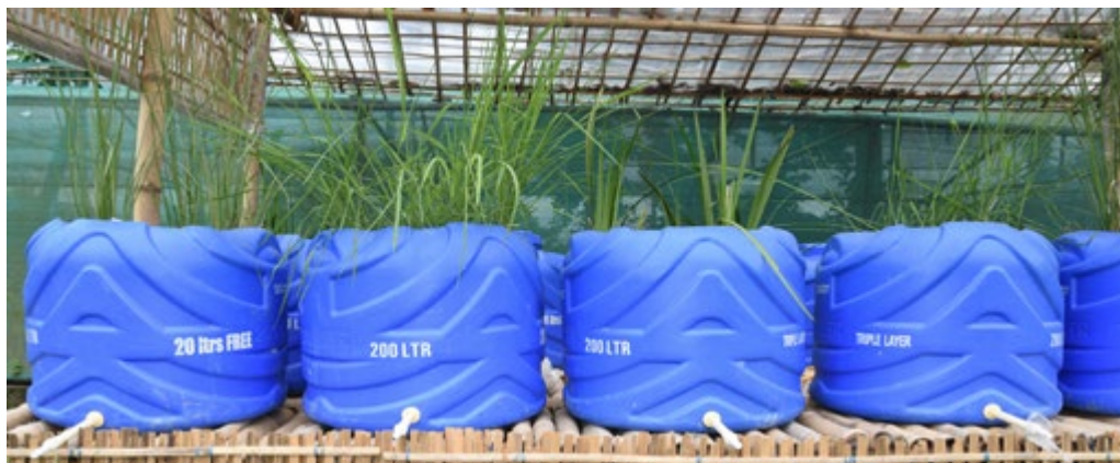
Fig. 8. Experimental microcosm study for determination of effluent removal with various wetland macrophytes
