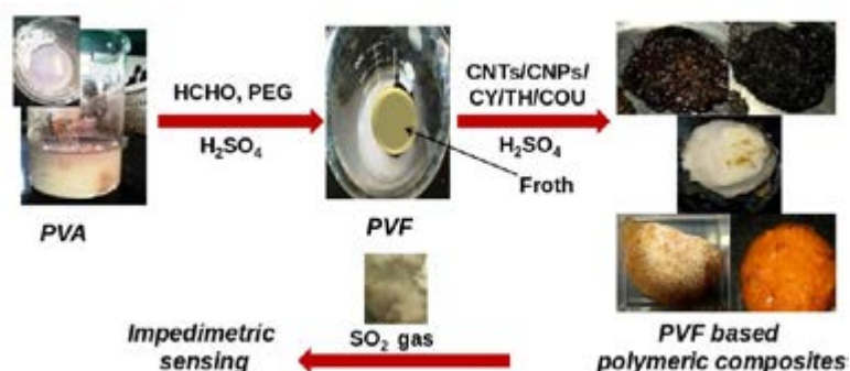
Fig.1 : Schematic representation of the \text{SO}_2 vapour detection system
